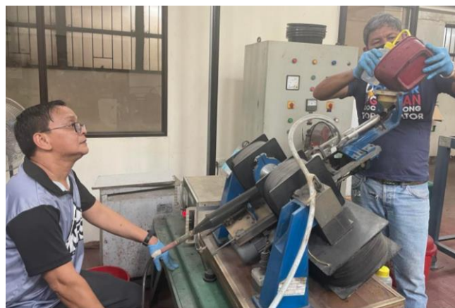
Fig. 4. Recovery of Iron from leaching tails using Davis Magnetic Tube
